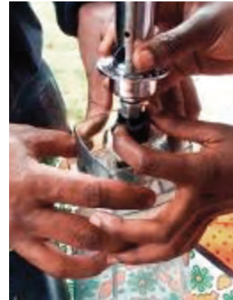
Figure 35.35: Fitting the blender to the bicycle.
