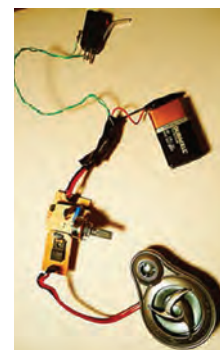
Figure 37.3: Oscillator circuit with 555 chip.
