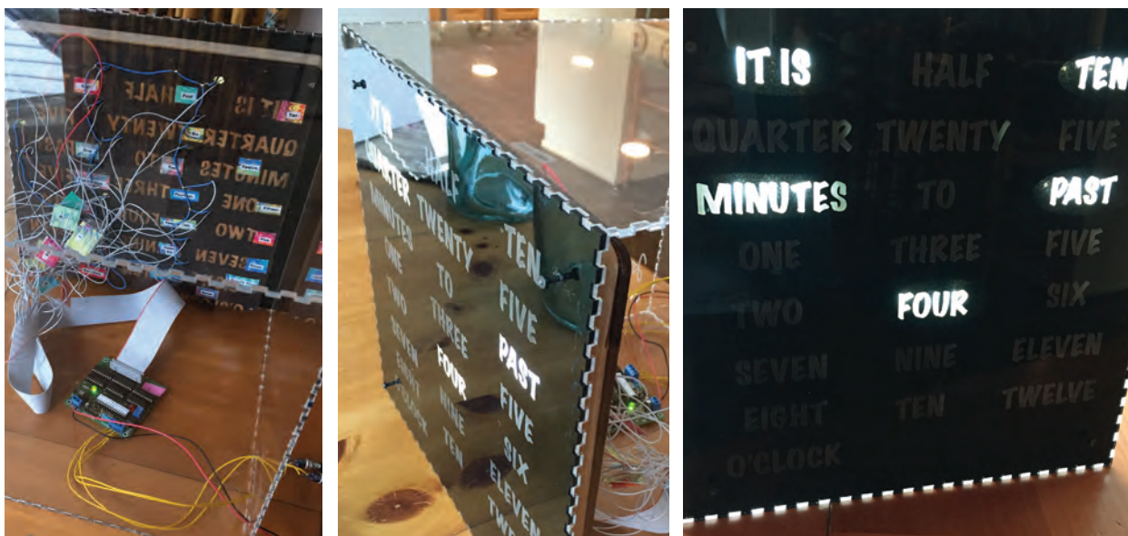
Figure 4.4: Transparent word clock enclosure design with marbled paper.
