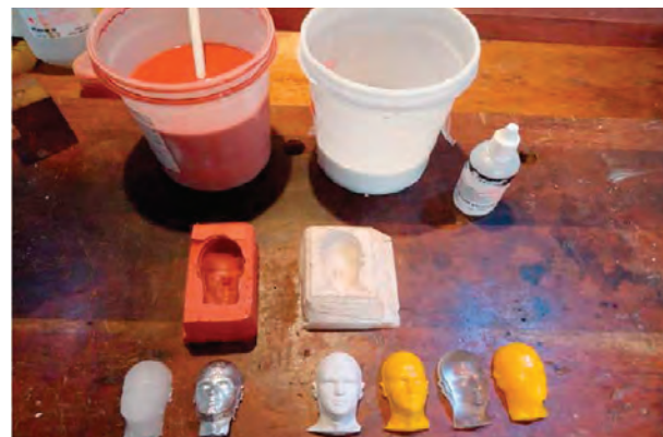
Figure 30.6: High-temperature molding (left) and low-temperature molding (right).
