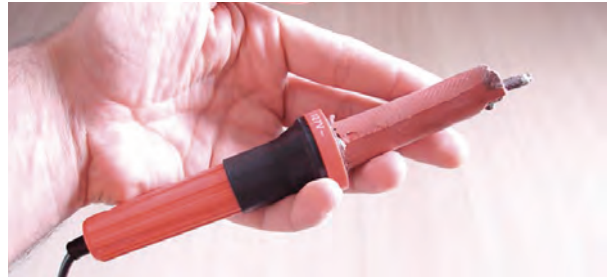
Figure 32.2: Silicone protector on the soldering iron.
