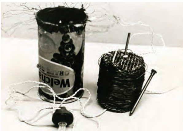
Figure 16.1: Tin-can radio design by Victor Papanek.
