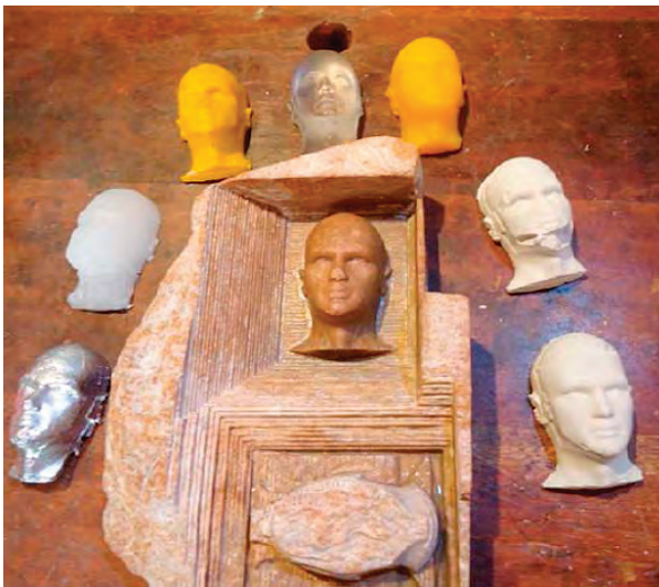
Figure 31.1: Objects of different materials cast from the same mold.
