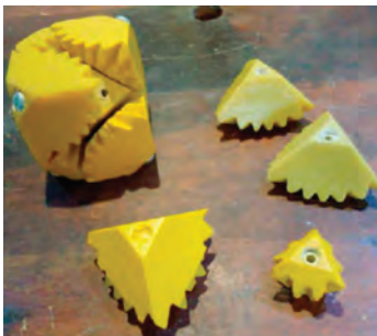
Figure 31.8: Gear cube parts made in a mold.
