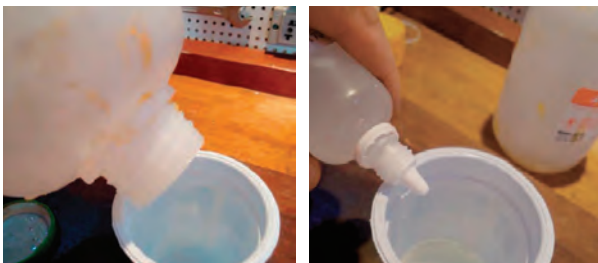
Figure 31.4: Pour pigmented resin in mold and remove finished workpiece when cured.
