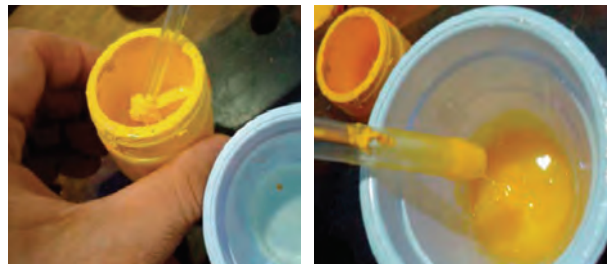
Figure 31.2: Pigment paste for resin. Figure 31.3: Add pigment to resin.
