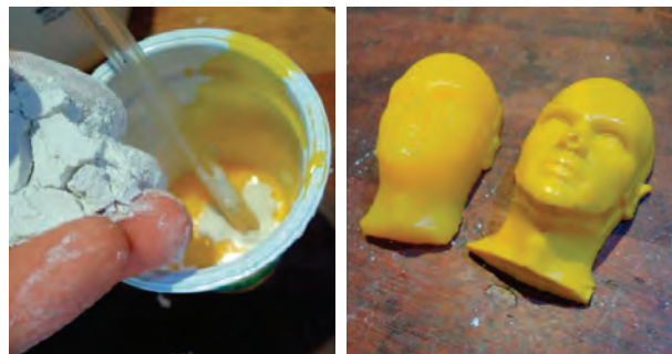
Figure 31.5: Adding talcum powder to resin mixture.
