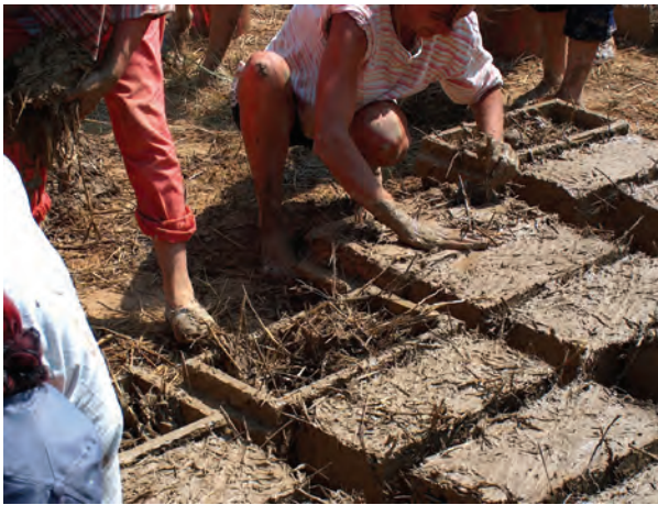
Figure 30.3: Making bricks in molds, a process still used today.
